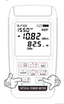
In the optical power meter mode, short press REF to switch the optical power unit (dB/dBm) and review the REF value. Long press this key to set the current power value as the new REF value, Short press Short press to switch measuring wavelengths, long press this key to activate wavelength recognition function.
