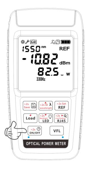
Short press to turn on the device, auto-off mode activated, if there is no button operation in 10 minutes, the instrument will shut down automatically.
