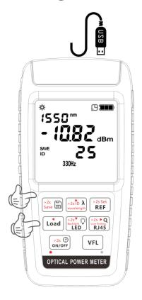
In testing mode, long press to save the currently measured data. The instrument can store 500 sets of data, and the storage sequence numbers will automatically accumulate in order. Excess data will not be saved unless previously saved data is deleted first.
